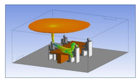
Figure 1: Distribution of aerosols emitted by an infected sneezing person inside a meeting room
