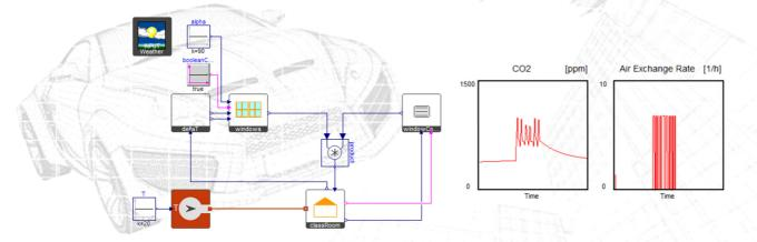
Figure 2 Dynamic room model of a classroom to optimise the ventilation control
